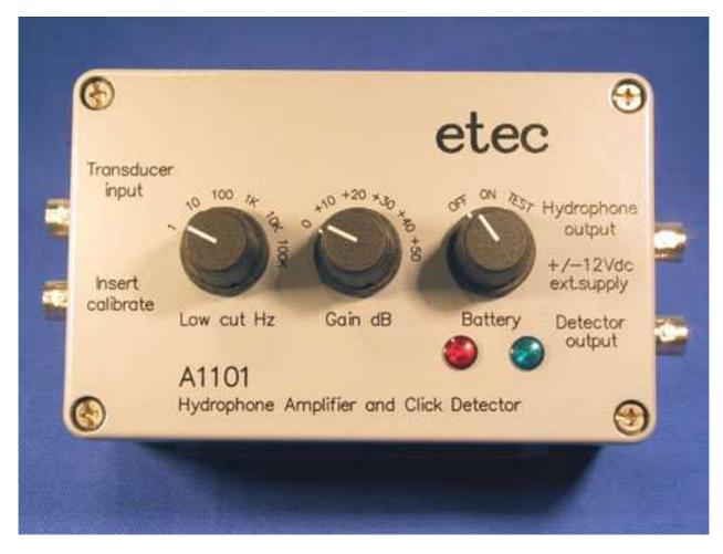
Hydrophone amplifier with batteries. Amplifier with build in 2 pcs. 9Volt PP3 batteris. This unit may also be powered by an external 12Volt battery or by a +/- 12Volt dual power supply.
