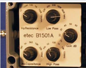
B1501 Hydrophone amplifier and cable driver with high- and low pass filters and buffered output. Two pcs. 9Volt square battery supply offers 18Volt supply and very high output signal level.
