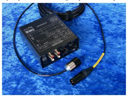
This unit is compatible with most any type of professional studio recording and reproduction equipment. We recommend the ZOOM type H4 handheld digital recorder to supplement this listening amplifier for recordings and documentation. This device will record the audible range 20hz to 20kHz.
