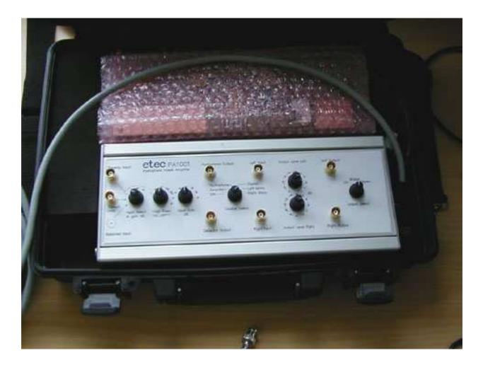
This amplifier is a stand alone unit with a power amplifier and a hydrophone reciever amplifier complete with buildin envelope or "click" detector and batteries and charger supplied all together in a watertight suitcase.
